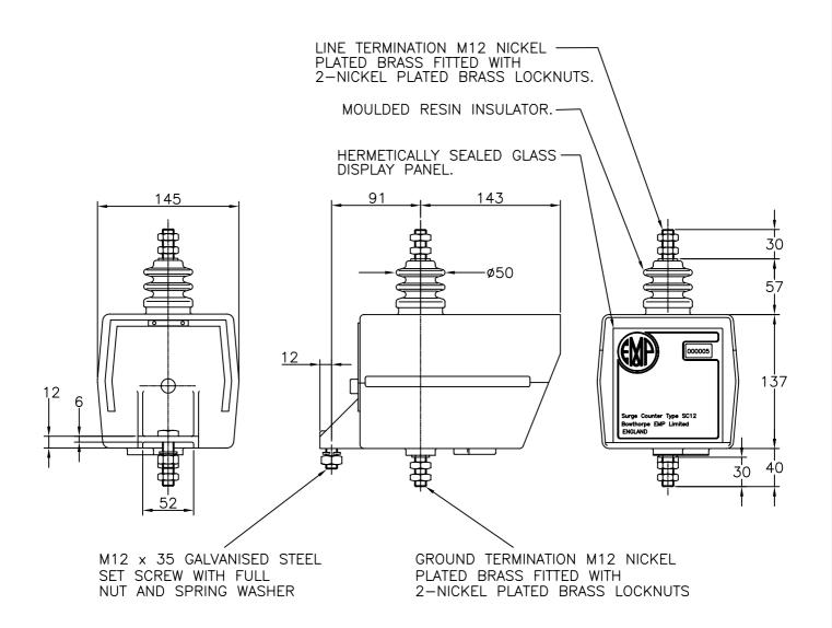
MAX TIGHTENING TORQUE FOR CONNECTIONS AND MOUNTINGS 40Nm
