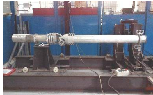
Cantilever/Bending test up to 5T/Axis
