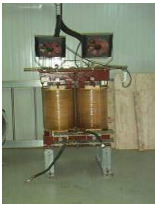
Short-circuit test up to 42kA/2Sec
