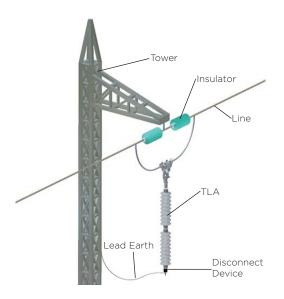
The number of the surge arresters installed on the tower depends on the tower geometry and configuration as well as the earthing impedance behaviour.
